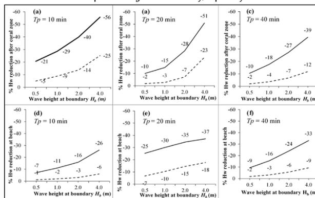
Figure 5: Marine flood mitigation potential of the coral reef on the idealized bed profile (Fig. 1a) with wave period. (a, b, and c) wave height reduction behind the reef and (d, e, and f) wave height reduction at the shore compared to the case without reef. Thick and dotted lines show the results for Manning's roughness of 0.25 and 0.1, respectively.  $H_b$  and  $T_p$  are the wave height and wave period at the generation boundary, respectively.
